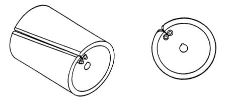
2) DRUM MARKS......are caused by the operator lowering the drum to the floor without forward traverse. These marks should be removed by cutting at a 45 degree angle to the mark. Cutting at the mark while maintaining the same path will only increase the mark depth and width.
